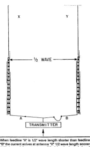
"B" the current arrives at antenna "X" 1/2 wave length sooner (180 degrees) than at antenna "Y" giving the "out of phase" end fire pattern.
