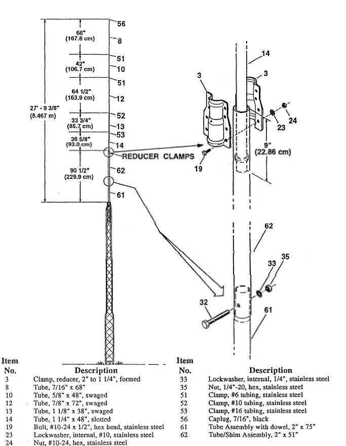
Figure 7 Vertical Radiator Assembly
