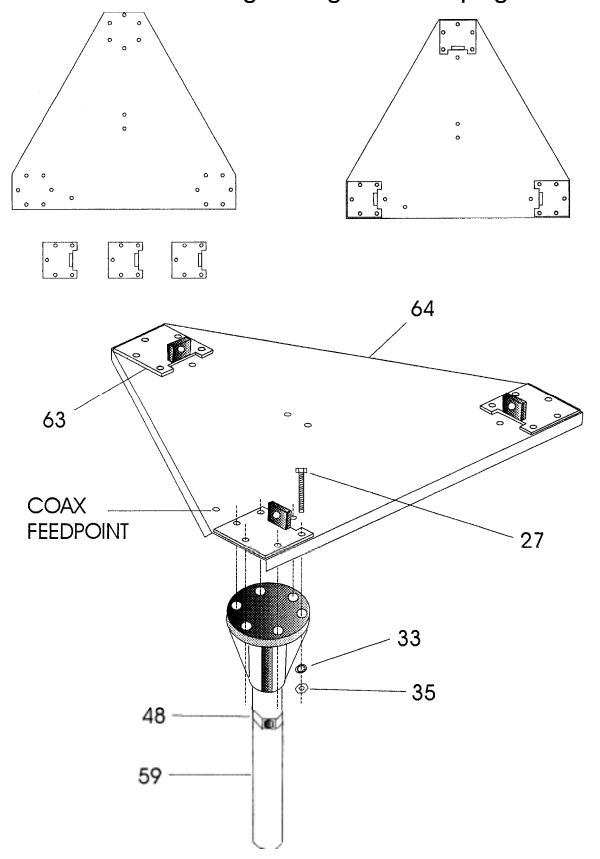
The tower plates inside the Hy-tower have been improved. The new plates are made from stainless steel, Install the lower plate as shown in the diagram, One X has been left out of the top section to allow for easy installment of the lower (larger) triangle. Install two spacers between the triangle tab and the tower leg,
